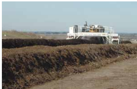
Figure 13.3. Turning a compost pile at a commercial facility. Photo by Alison Jack.
