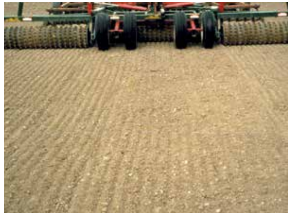
b) Stage 2: Soil is packed and pulverized to make a fine seedbed.
