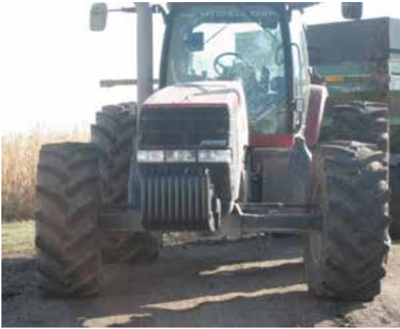
Figure 15.10. A tractor with wide wheel spacing to fit a controlled traffic system.
